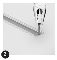
Screw the bolt down until it stops. Use a pair of pliers to grip the bolt, pull to raise one end of the product.
